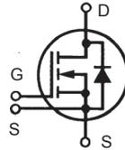
$$\begin{aligned} V_{DSS} &= 500 \text{ V} \\ I_{D25} &= 80 \text{ A} \\ R_{DS(on)} &= 55 \text{ m}\Omega \\ t_{rr} &\leq 250 \text{ ns} \end{aligned}$$
