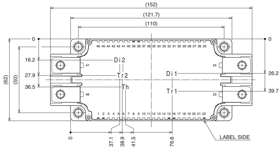
Each mark points the center position of each chip. Tr\*: IGBT, Di\*: FWDi, Th: NTC thermistor
